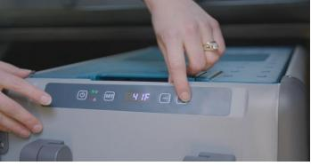
Adjust to desired temp using plus and minus buttons and push "Set".
